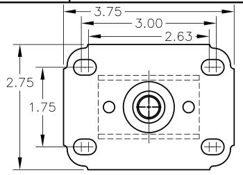
NOTES: LOAD RATING = 125 LBS. WHEEL = GRAY TPR RUBBER TREAD ON GRAY POLYPROPYLENE HUB WITH DELRIN BEARING
